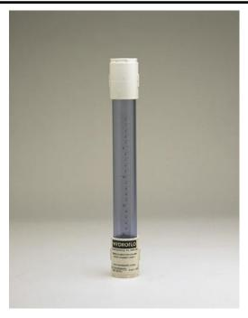
NIKKISO HydroChek<sup>™</sup> Loss-In-Volume flow verification systems provide a compact, cost effective solution for applications requiring periodic flow monitoring or pump calibration. HydroChek Columns are used as precision, volumetrically calibrated pump suction vessels. By calculating the specific volume of process fluid displaced per unit time, they verify the performance of any pump in its specific application.
